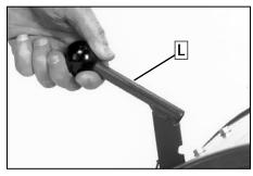
Figure 2-8: Put lever in second notch.
